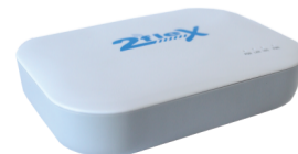
ONU EPON Bridge
